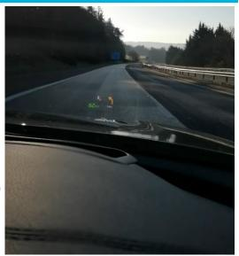
things such as current speed, Sat Nav directions, warning messages and blindspot notifications.
